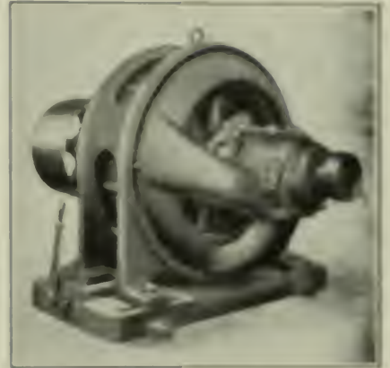
FIG. 1. A NEW BELT-DRIVEN ALTERNATOR
